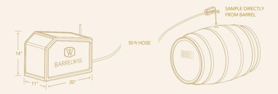
The BarrelWise FS1 is a cloud-connected free SO<sub>2</sub> analyzer that automates sample acquisition, analysis and data collection.
